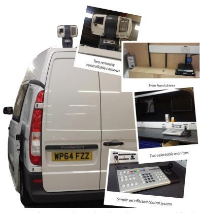
The Van is a High Top Mercedes Vito van with a viewing room separate from the front drivers area and a separate area for battereies and Hard drives
